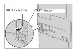
Press the <RESET> button back to the depressed position.
