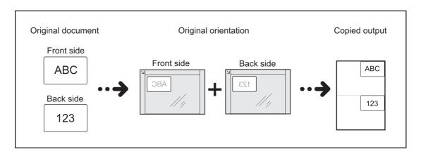
**1** Specify the orientation of the document in [Original Orientation] on the [Layout Adjustment] screen.
