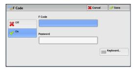
**8** Select the [F Code] box, and enter the F Code using the displayed keyboard or the numeric keypad.
