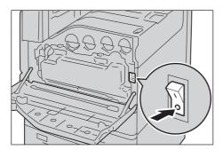
5. Press the <TEST> button on the power plug to turn off the ground fault interrupter. Check if the power lamp turns off. If the lamp turns off, it means that the ground fault interrupter circuit works properly.
