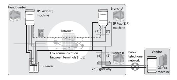
IP Fax (SIP) can be configured with SIP server and VoIP Gateway. The functions of the devices are as follows:
