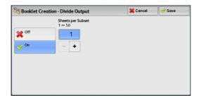
**2** Specify the number of sheets in each subset, using [+] and [-] or the numeric keypad.
