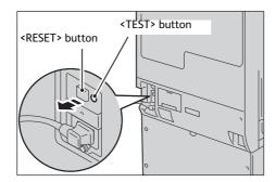
6. Press the <RESET> button back to the depressed position.
