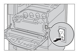
**5** Press the <TEST> button lightly with a sharp edge such as a pen tip. The depressed <RESET> button will stick out again.
