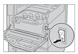
5. Press the <TEST> button lightly with a sharp edge such as a pen tip. The depressed <RESET> button will stick out again.
