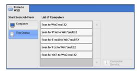
**2** Computer names and 5 processing methods are displayed in the [List of Computers]. Select destination from the list in accordance with the intended use.
