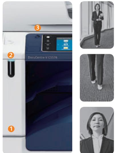
**1** This incredible technology uses an infrared pyroelectric sensor to monitor thermal changes in the vicinity of the device, to detect a person approaching.
