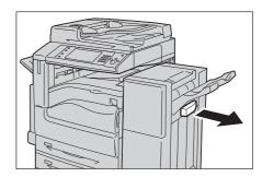
Install the tray attachment onto the middle of the finisher tray as shown in the diagram.
